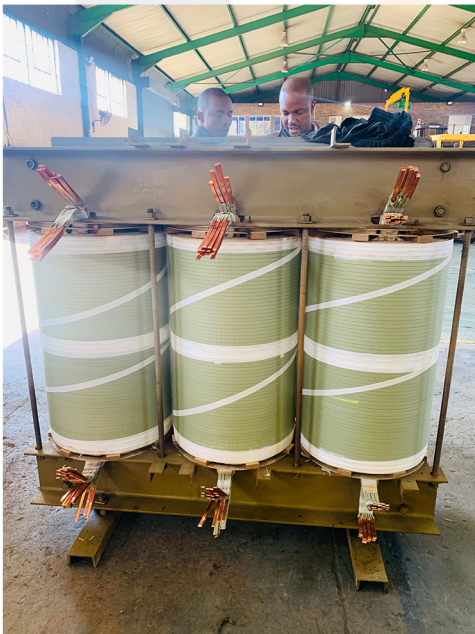
3150kVA 11/0.4kV Transformer - Rewind End User: South Africa Bureau of Standards
