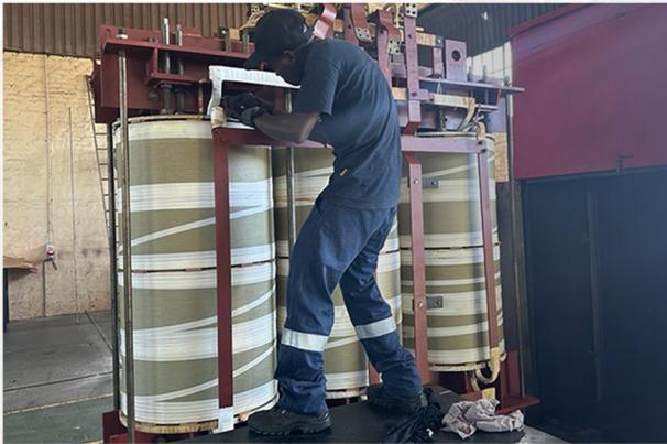
5MVA Active Part - Tanking
